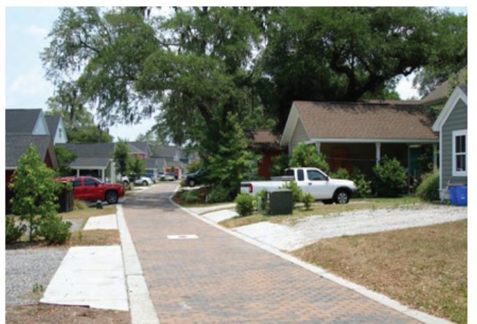
Sustainable technologies like the pervious paving above blend with old oak trees in this green development. Photo credits Southeast Watershed Forum.
