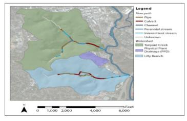
FIGURE 2. This map shows the flow path of the Campus Watershed's water bodies, indicating which portions are piped or in culverts and which are daylighted.
