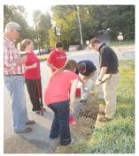
PHOTO 6B. Flow in dry weather in a stormwater pipe suggests sewage leak.
