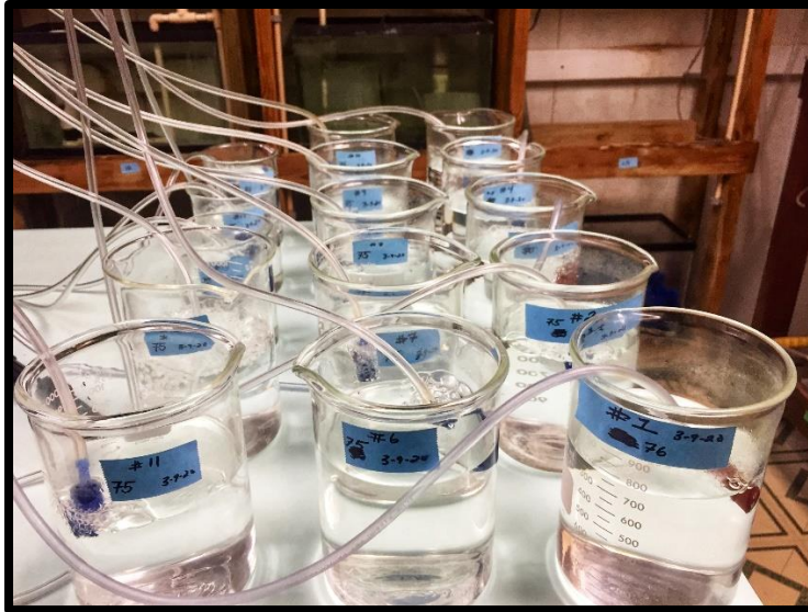
Figure 2. Photo showing neonate acclimation chambers where neonates were grown into 7-8-day old test organisms.
