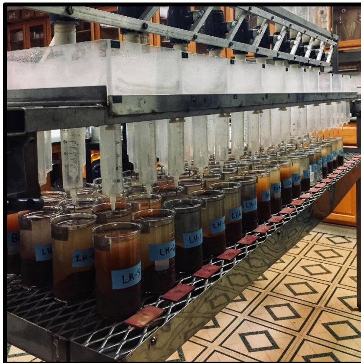
Figure 3. Photo showing setup of static renewal system for renewal of overlying water.
